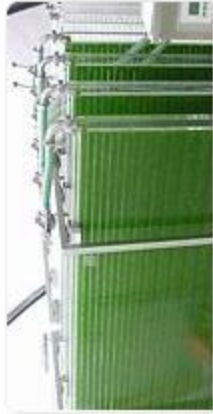
Glass Tubular Photobioreactors for cultivation of algae ...
